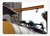
the loads generated by a cable type multi-span horizontal lifeline system. In addition, rigid systems eliminate sag and deflection, reducing the overall fall clearance needed below the work area.
